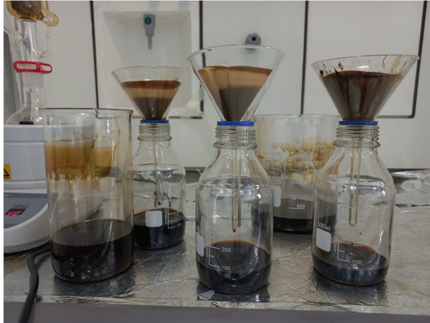
Figure 3-3. Filtration of asphaltene using filter paper
