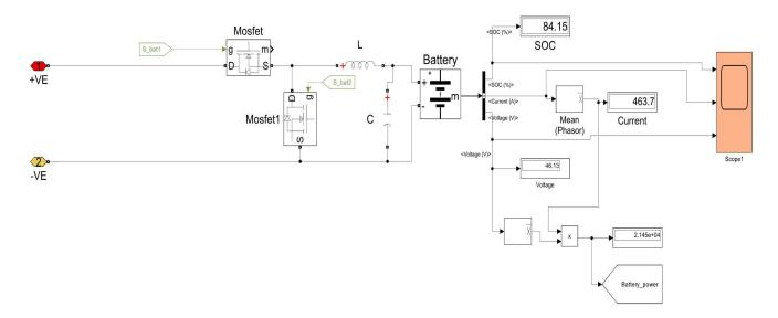
Figure .3.10 battery energy storage system
