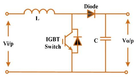
Figure .3.6 illustration of the circuitry for a DC-DC boost converter
