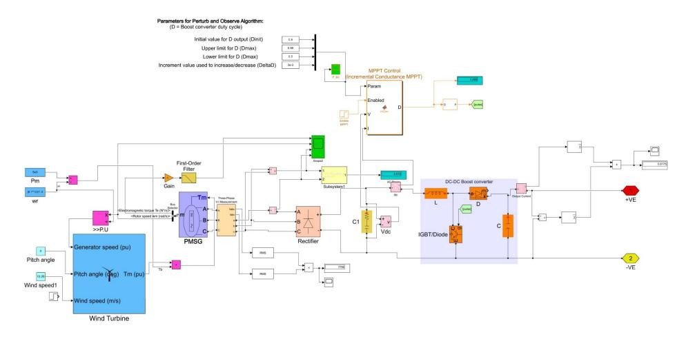
Figure .3.8 simulation model of wind turbine
