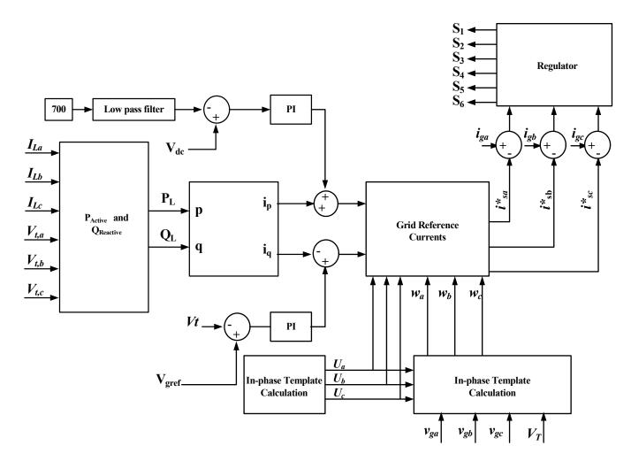
Figure 3.12. Control algorithm based on the power balance (PB) theory.
