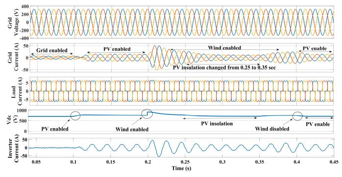
Figure .5.3 simulation results of the grid synchronization of the microgrid system
