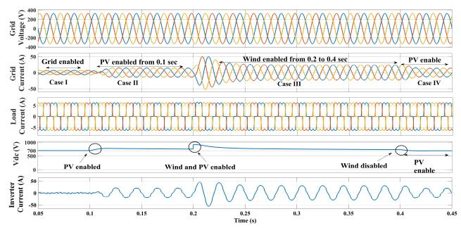
Figure .5.1 simulation results for grid voltage and current, load current, DC link capacitor, and inverter current
