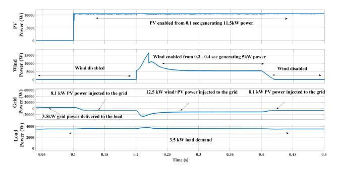
Figure .5.2 power generation from the renewable energy sources (PV and Wind)
