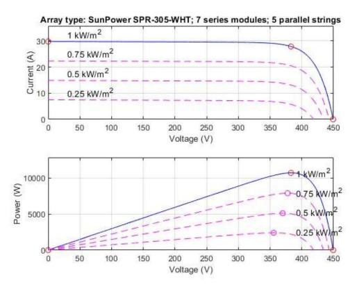
Figure .3.5 VI characteristic waveform and MPP plot of the PV system
