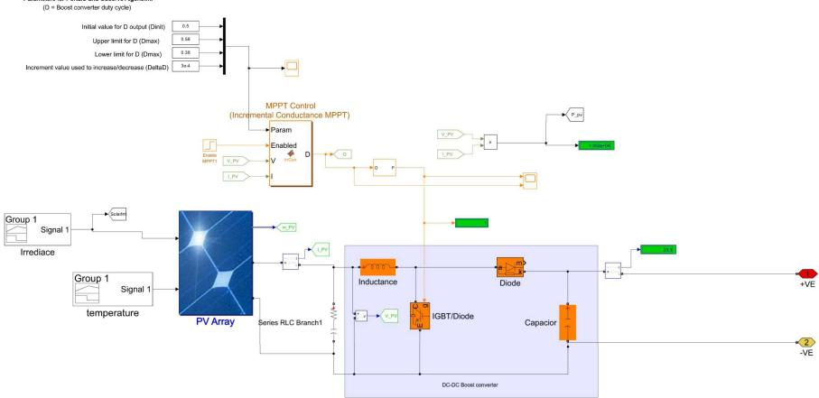
Figure 3.3-simulation model of the PV system
