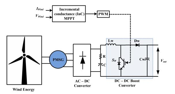
Figure .3.7 schematic architecture of wind turbine (PMSG) with its MPPT control algorithm[4]
