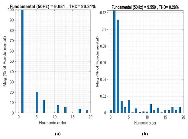
Figure 5.5: THD analysis of phase a grid current
