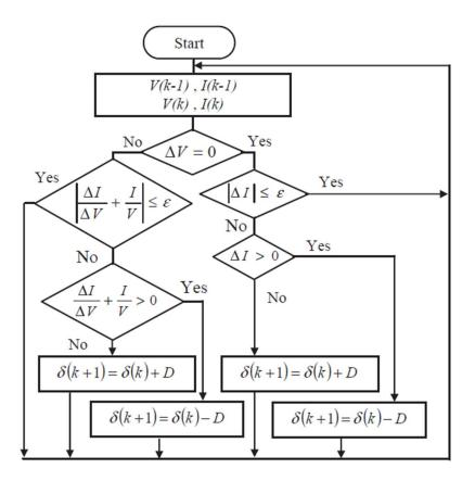
Figure .3.9 incremental conductance MPPT flow chart
