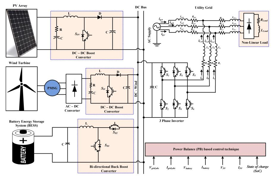
Figure .3.1 schematic diagram of MG with its boost converter and control operation[4].
