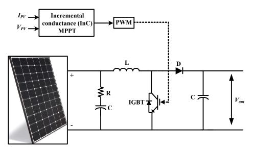
Figure .3.4 solar arrays with their boost converter and MPPT algorithm[4]
