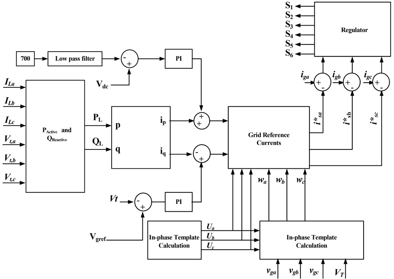
Figure 3.12. Control algorithm based on the power balance (PB) theory.
