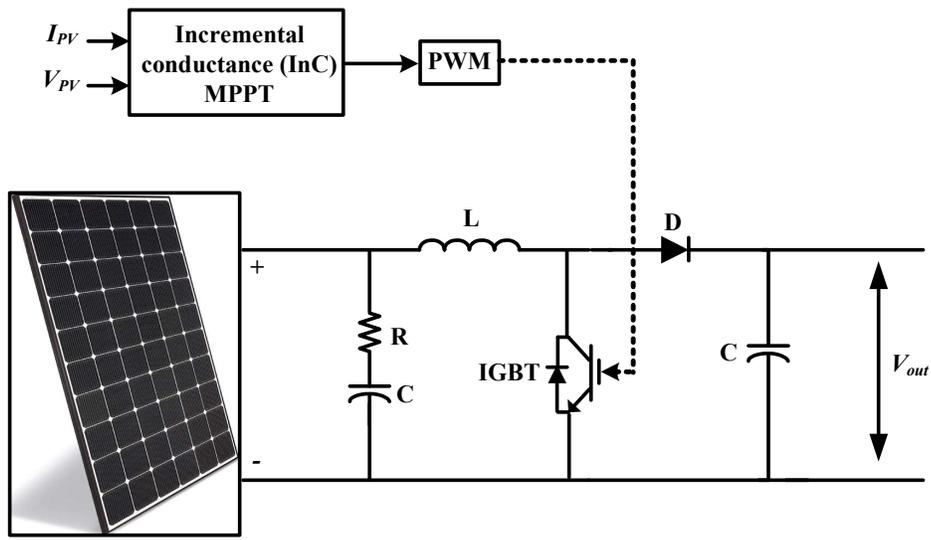
Figure .3.4 solar arrays with their boost converter and MPPT algorithm[4]
