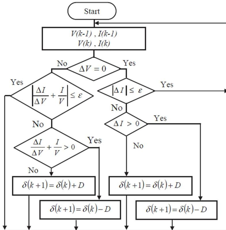
*Figure .3.9 incremental conductance MPPT flow chart*
