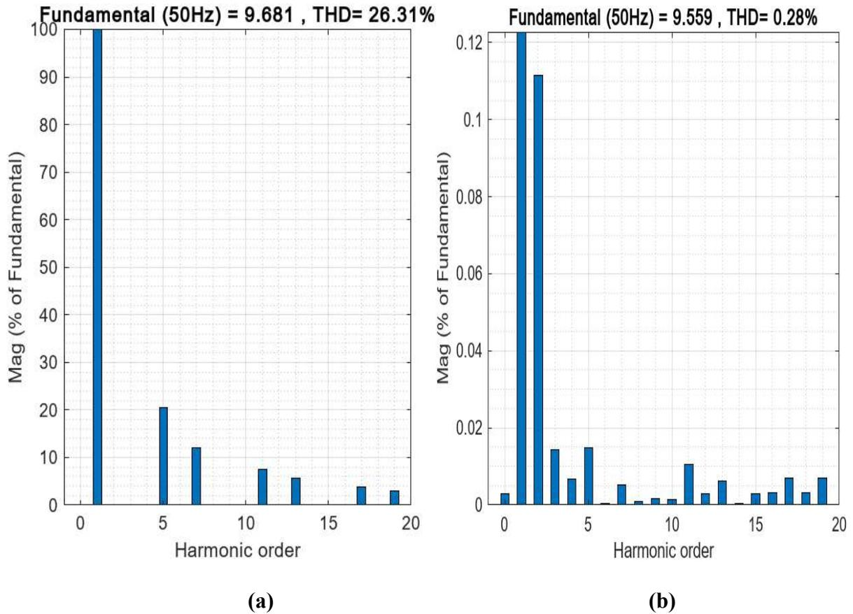
**Figure 5.5: THD analysis of phase a grid current**
