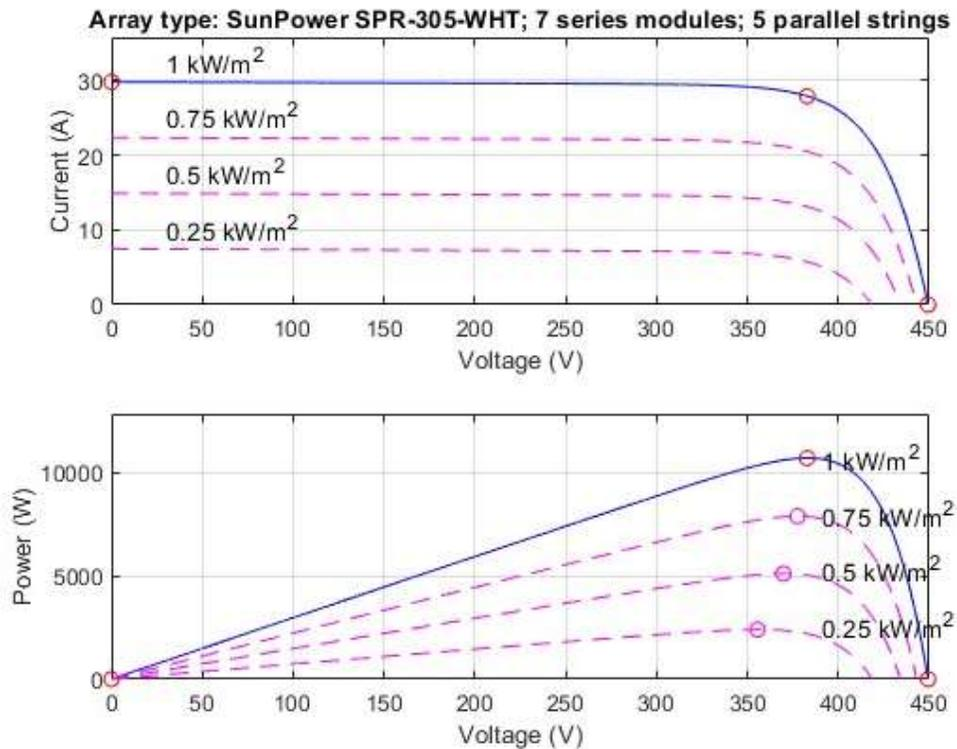
Figure .3.5 VI characteristic waveform and MPP plot of the PV system
