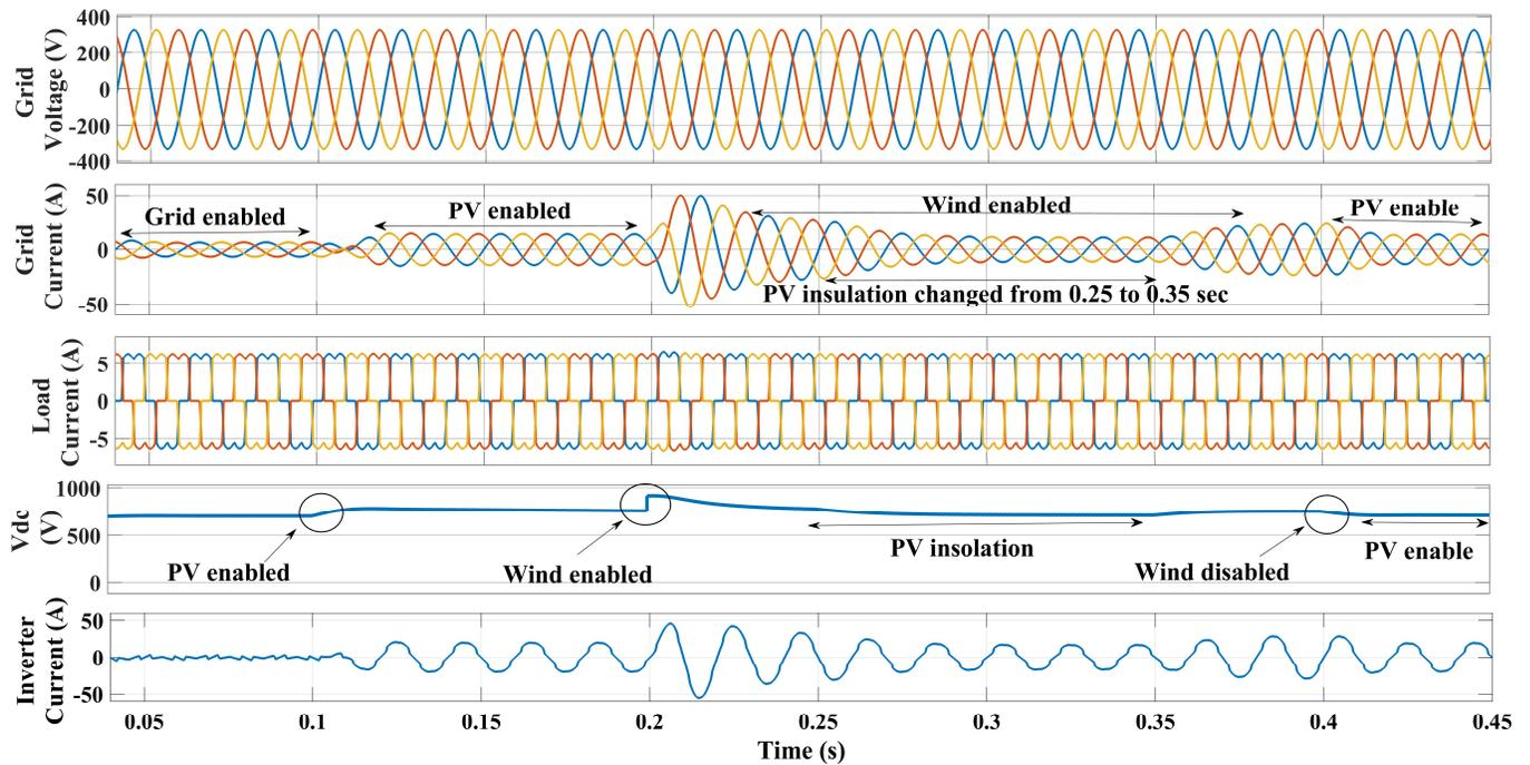
**Figure .5.3 simulation results of the grid synchronization of the microgrid system**
