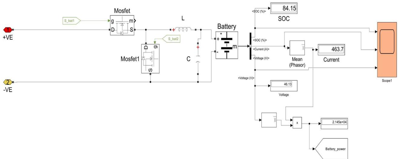
**Figure .3.10 battery energy storage system**
