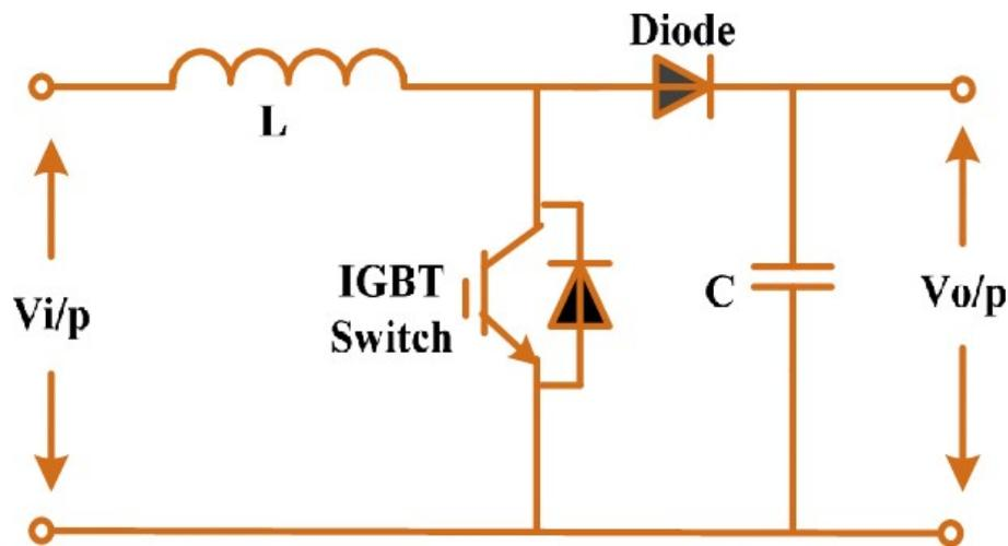
*Figure .3.6 illustration of the circuitry for a DC-DC boost converter*
