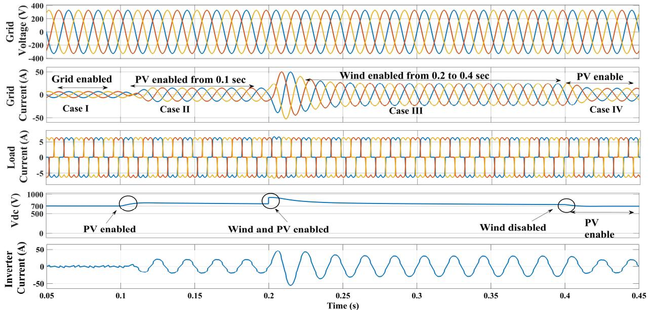
**Figure .5.1 simulation results for grid voltage and current, load current, DC link capacitor, and inverter current**
