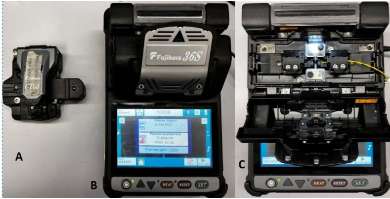
Figure 8. Special diamond cleaver (A) and Fujikura 36S Splicing machine (B). Splicing process of fabricated ball resonator to the pigtail (C).
