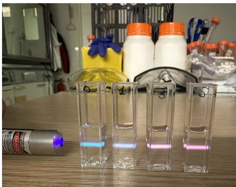
Figure 20. The image of the emitting light changes from green-blue to red with increasing concentration TC
