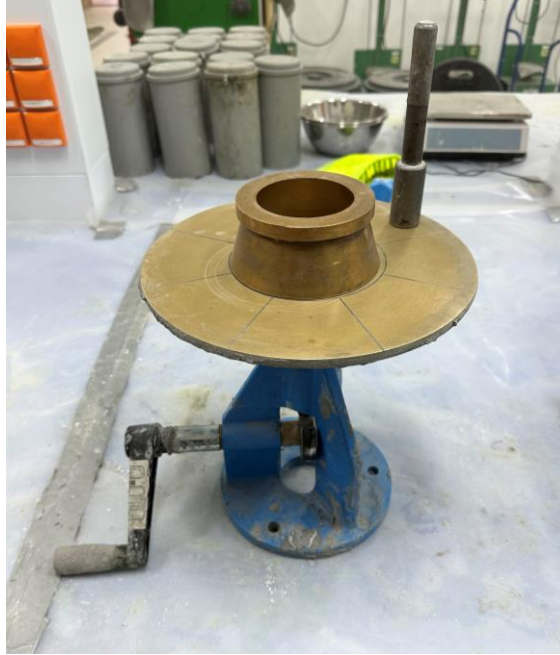
Figure 3.14. Flowability measurement equipment
