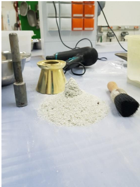
Figure 3.7. The SSD condition of WGS and pycnometer apparatus
