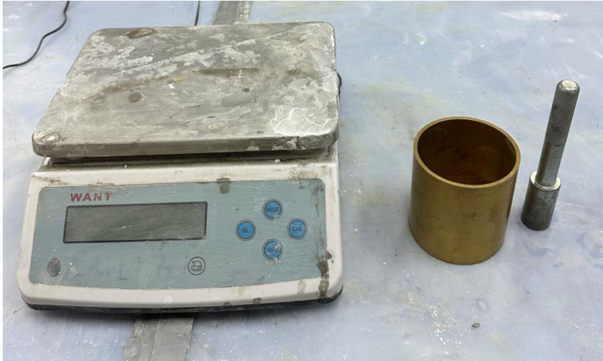
Figure 3.15. Air content measurement equipment
