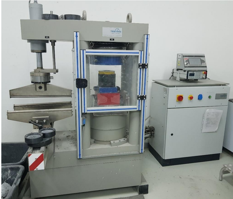
Figure 3.16. Compressive strength measurement apparatus
