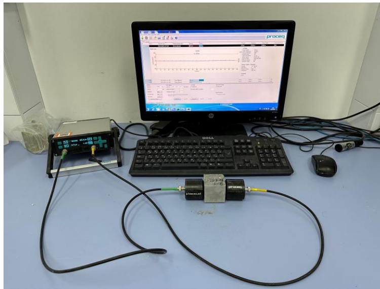
Figure 3.19. UPV measurement equipment
