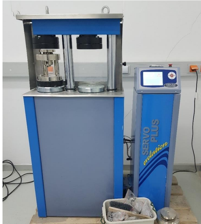
Figure 3.17. Flexural strength measurement apparatus
