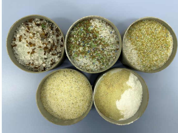
Figure 3.5. #8, #16, #30, #50 and #100 sieves size WGS
