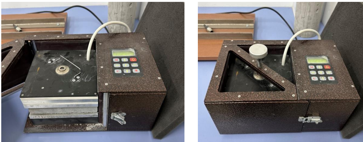
Figure 3.18. Thermal conductivity measurement device
