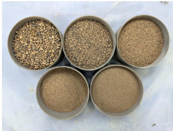
Figure 3.6. #8, #16, #30, #50 and #100 sieves size RS
