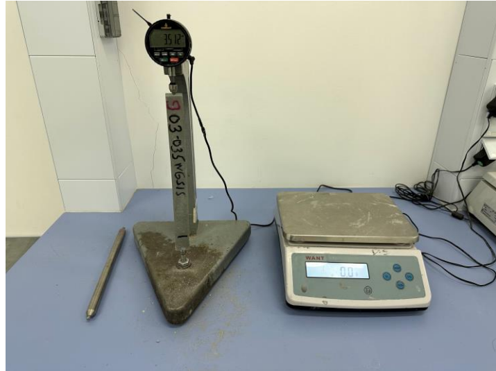
Figure 3.22. Devices for drying shrinkage test
