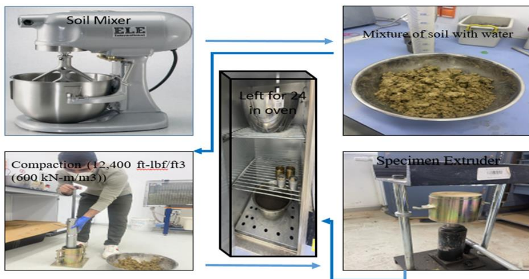
Figure 4-1 The process of proctor test for determination of maximum dry density.
