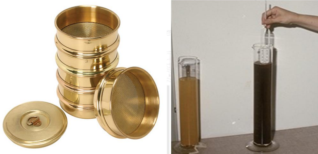
Figure 4-3 Sieve and hydrometer analyses
