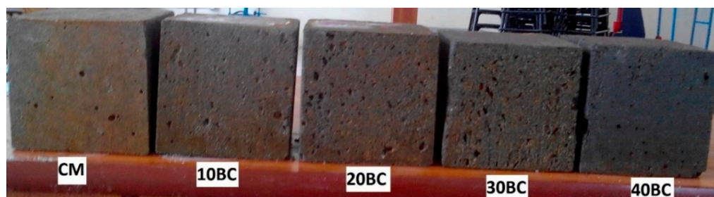
Figure 16. Specimens after immersion in hydrochloric acid.
