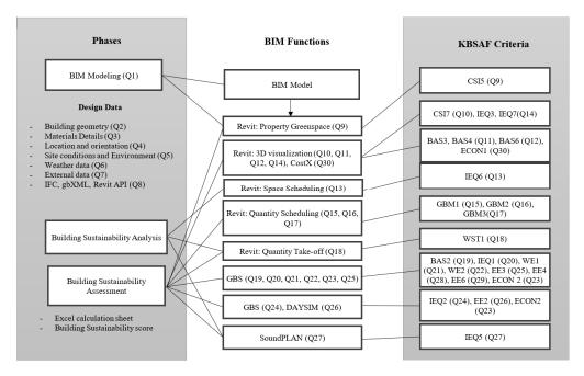
**Figure 2.** Conceptual Framework for BIM-based Building Sustainability Assessment in Kazakhstan (BIM-KBSAF).
