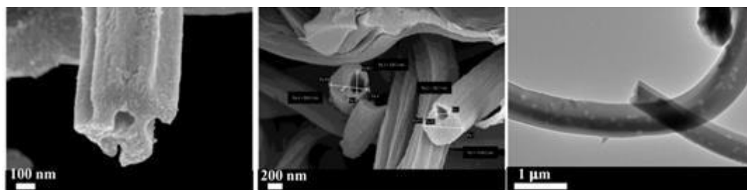
Figure 1. (a), (b) SEM image of HCNF, (c) TEM image of HCNF
