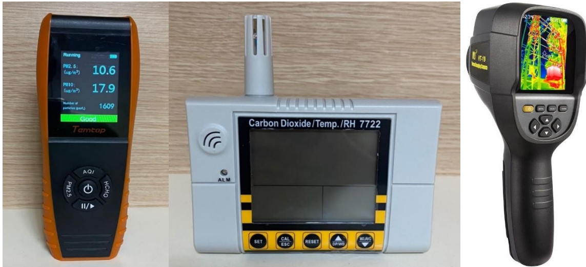
Figure 9. PM meter, CO 2 sensor, and thermal camera.
