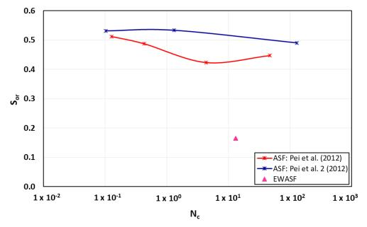
Figure 3. Comparison of capillary desaturation tendency of hybrid EWASF with conventional ASF.
