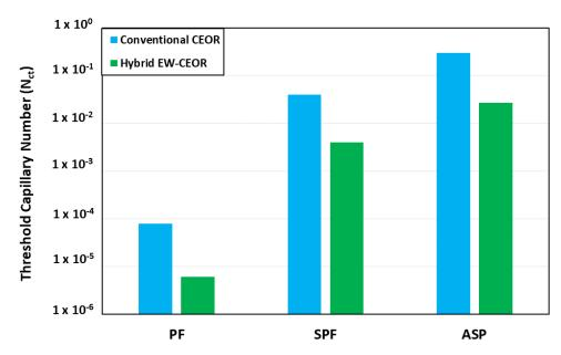
**Figure 7.** Comparison of threshold capillary numbers of hybrid EW/CEOR methods with conventional ones.
