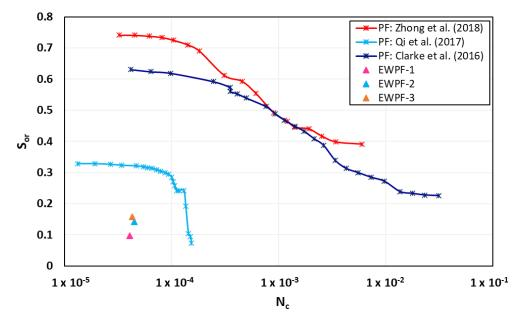
Figure 4. Comparison of capillary desaturation tendency of hybrid EWPF with conventional PF.
