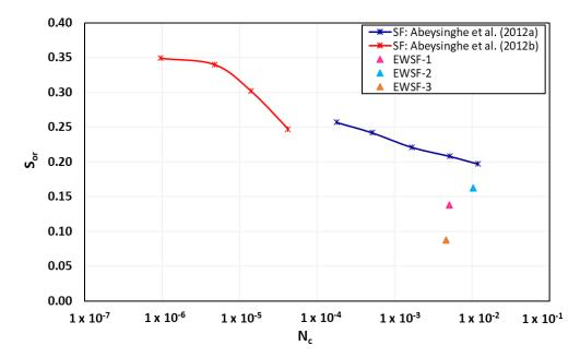
Figure 2. Comparison of capillary desaturation tendency of hybrid EWSF with conventional SF.
