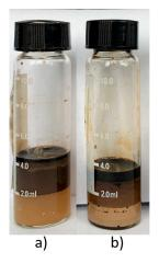
**Figure 1.** Results of phase behavior study for (**a**) EW-surfactant solution and (**b**) EW-surfactant solution with addition of 1 wt% alkali.
