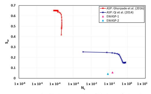
**Figure 6.** Comparison of capillary desaturation tendency of hybrid EWASP flooding with conventional ASP flooding.
