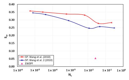
Figure 5. Comparison of capillary desaturation tendency of hybrid EWSPF with conventional SPF.
