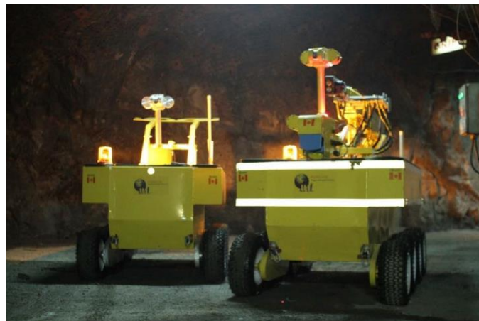
Figure 8. Robot system developed for geospatial mapping (After Baiden, 2016).
