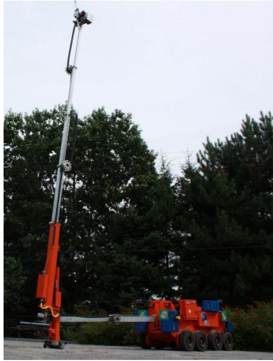
Figure 9. The robot system built by Penguin Automated Systems with extended arm for hang-up removals (After Baiden, 2016).
