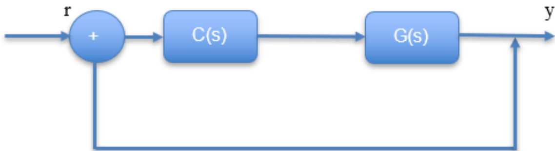
Figure 3.2.1 : Block diagram of a closed-loop control of a roll angle transfer function using PID controller
