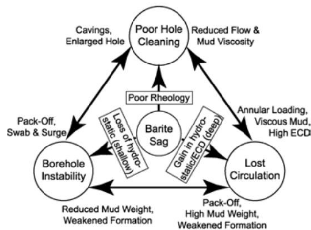
Figure 2. Problems associated with barite sag; borehole instability, poor hole cleaning [5].
