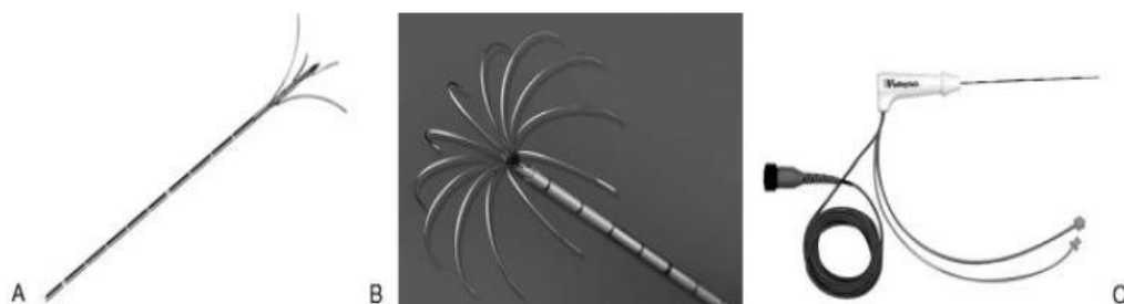
Figure 2.2 (A) 14-Gauge multitined StarBurst Talon RFA device (photo courtesy of Angio Dynamics). (B) 14-Gauge LeVeen needle showing 12 retractable electrodes
