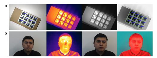
**Figure 6.** (a) Left to right: the visual image with identified ArUco markers; the original thermal image; a grayscale version of the thermal image; and a complement of the grayscale image with identified ArUco markers. (b) Left to right: the original visual image; the original thermal image; the result of aligning the visual image with it's thermal pair; and the result of replacing the red channel of the visual image with the red channel of the thermal image.
