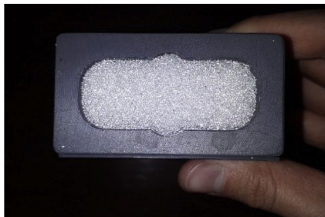
Fig. 4. Synthetic core in the PVC core holder.
