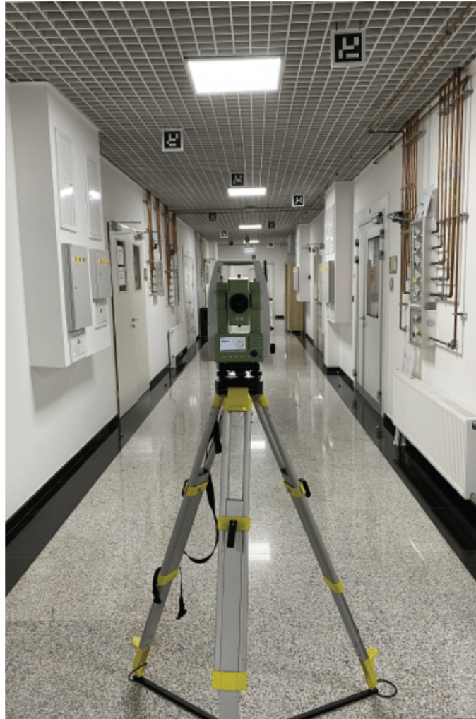
Figure 3-2: ArUco markers attached to the ceilings of the testbed and calibrated
