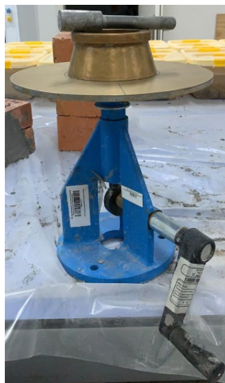
Figure 3.6: Apparatus for determination of flow of hydraulic cement mortar.
