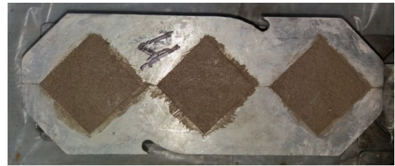
Cubic samples for Compressive strength test
