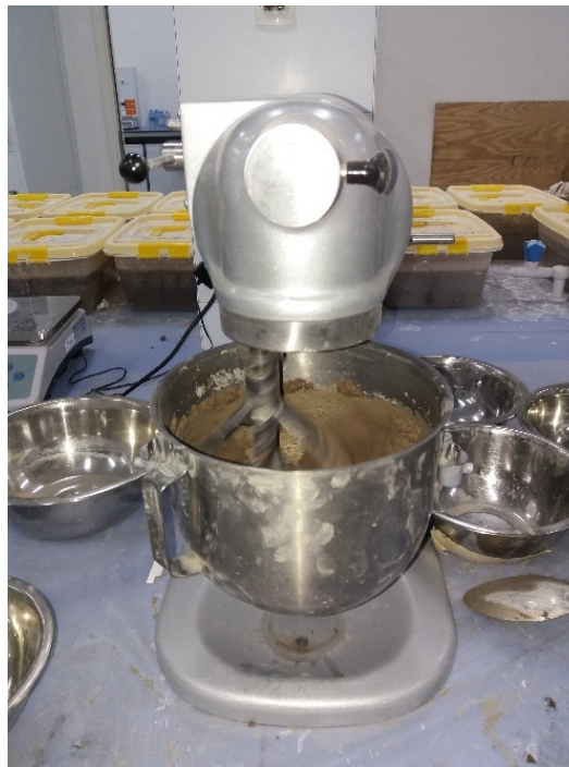
Figure 3.3: Mortar mixing with a Hobart 4.7-liter mixer.
