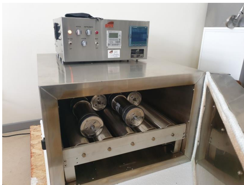
Figure 31. OFITE roller oven used in the static adsorption test
