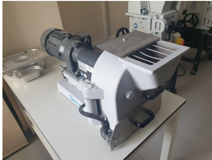
Figure 24. Disk chipper Retsch DM200 for crushing sandstone chunks
