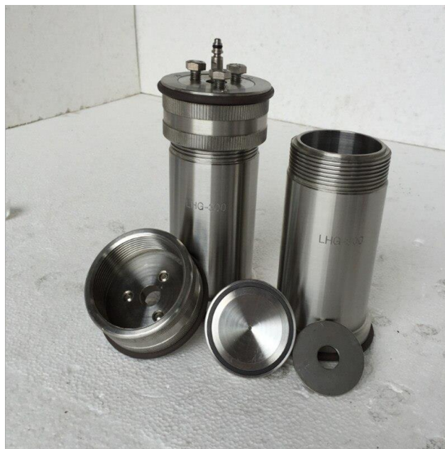
Figure 30. Ageing cells used for mixing in static adsorption test
