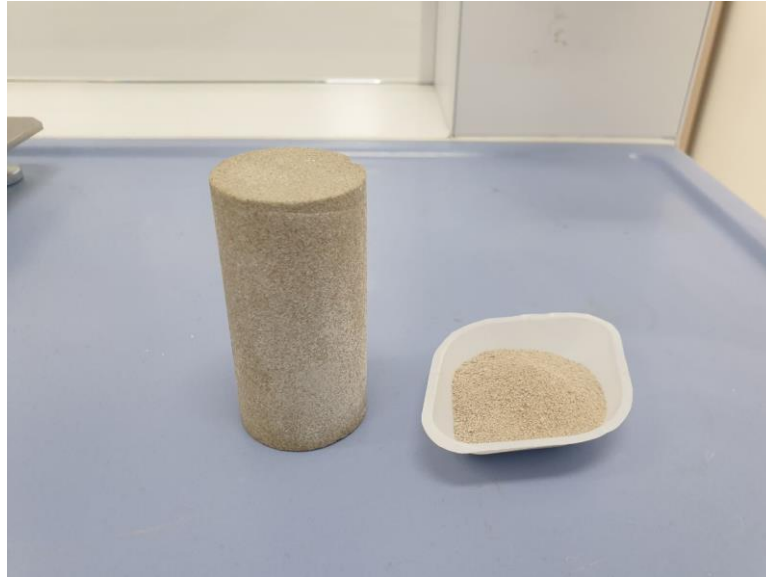
Figure 21. Core sample and sand powder used for adsorption tests
