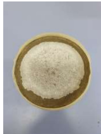
Figure 3.17: Development of salt crystallization during drying in wetting-drying cycles
