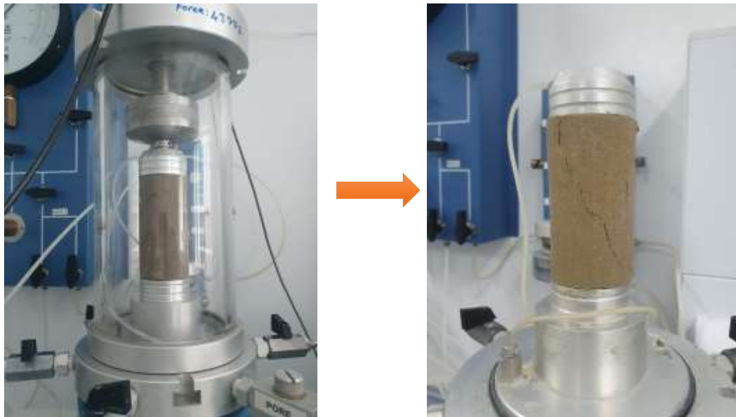
Figure 3.12: UCS test of the soil specimen
