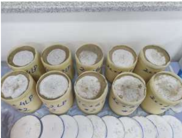
Figure 3.17: Development of salt crystallization during drying in wetting-drying cycles
