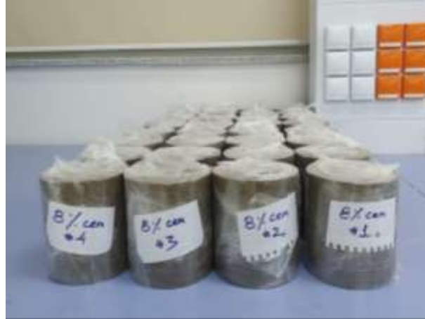
Figure 3.11: The cylindrical soil specimen cured in the sealed conditions
