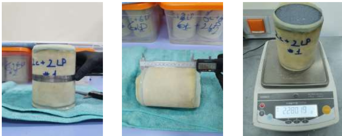
Figure 3.15: 3-D swell measurements
