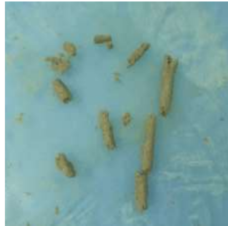
Figure 3.9: Determination of PL
