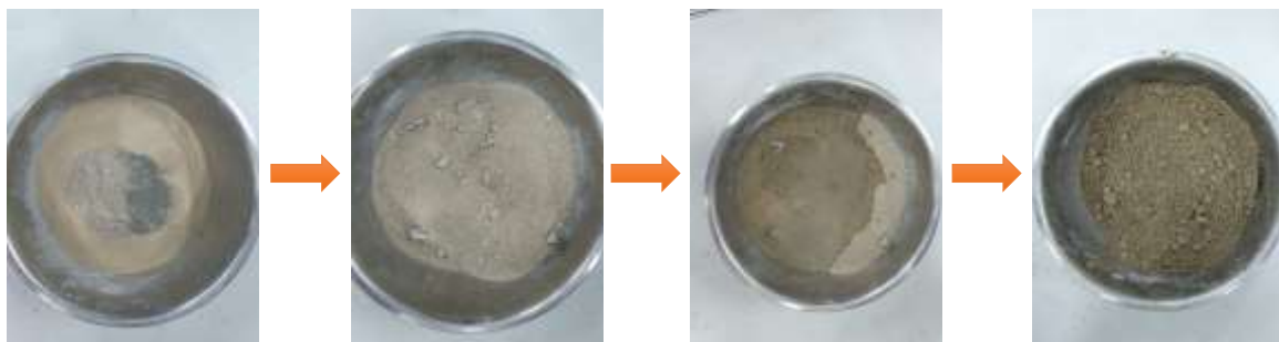
Figure 3.10: Soil-stabilizer mixing at the OMC
