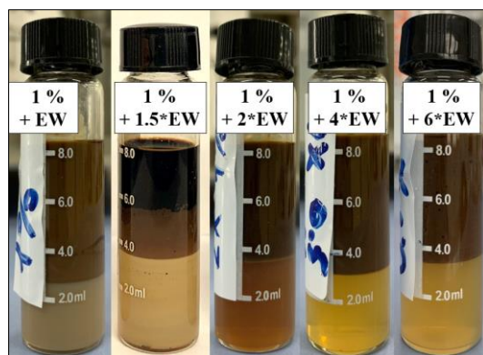
Figure 27. Phase behavior test at 80 °C for \text{Na}_2\text{CO}_3 concentrations of 1% of the aqueous phase with 1.5, 2, 4, 6 times diluted EW
