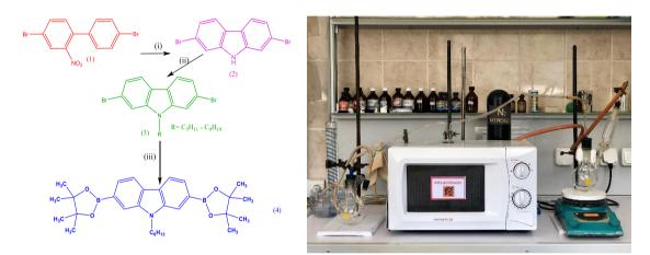
The use of a microwave flow reactor allowed to avoid a reducing of the microwave synthesis efficiency by increasing the amount of reagents and obtaining a bigger amount of product (2), (3), (4).
