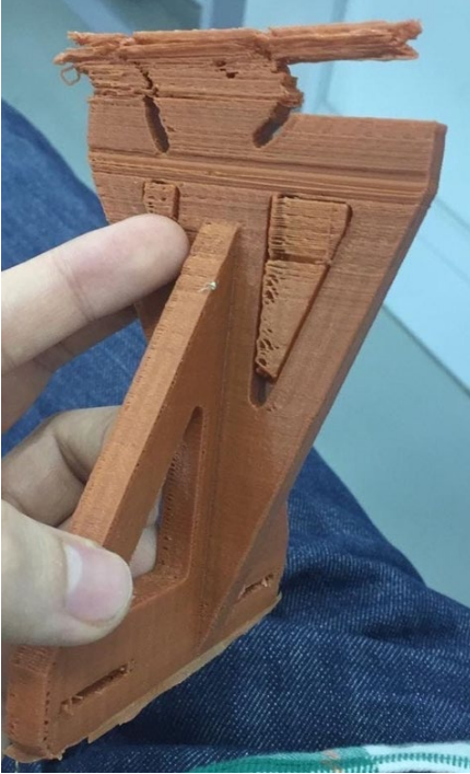
Fig.19 Unsuccessful sample of the frame design#2.
