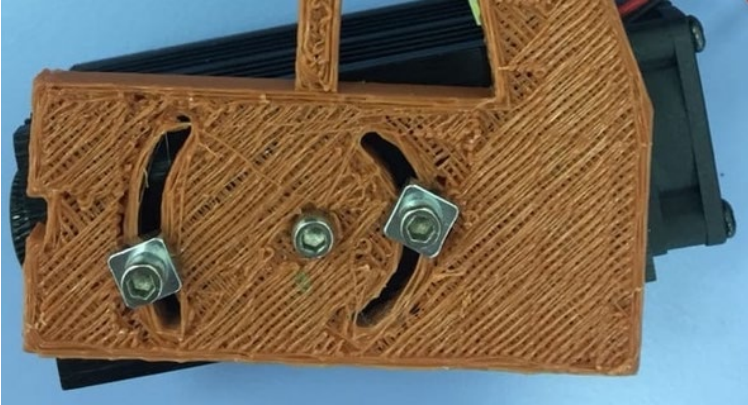
Fig.20. Rotation part of the frame
