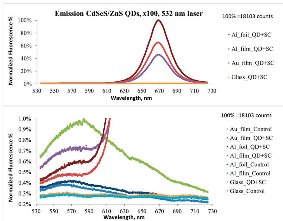
Fig. 3. Averaged Normalized Fluorescence Emission spectra of CdSeS/ZnS QDs with single bacterial cells (QD + SC) and of control (just SC) on various substrates, obtained with 532 nm laser excitation wavelength and  $\times 100$  objective. Maximum intensity for averaged spectrum QD + SC on Al foil is set as 100% (18,103 counts).
