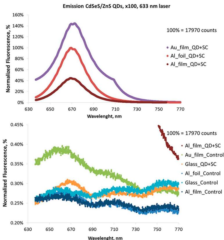
**Fig. 2.** Averaged Normalized Fluorescence Emission spectra of CdSeS/ZnS QDs with single bacterial cells (QD + SC) and of control (just SC) on various substrates, obtained with 633 nm laser excitation wavelength and  $\times 100$  objective. Maximum intensity for averaged spectrum QD + SC on Al foil is set as 100% (17,970 counts).
