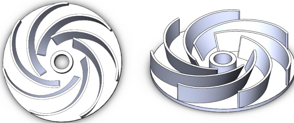
Figure 10. CAD models of 7-bladed impeller with Variable Blade Inlet Angle, top view (left) and isometric view (right).
