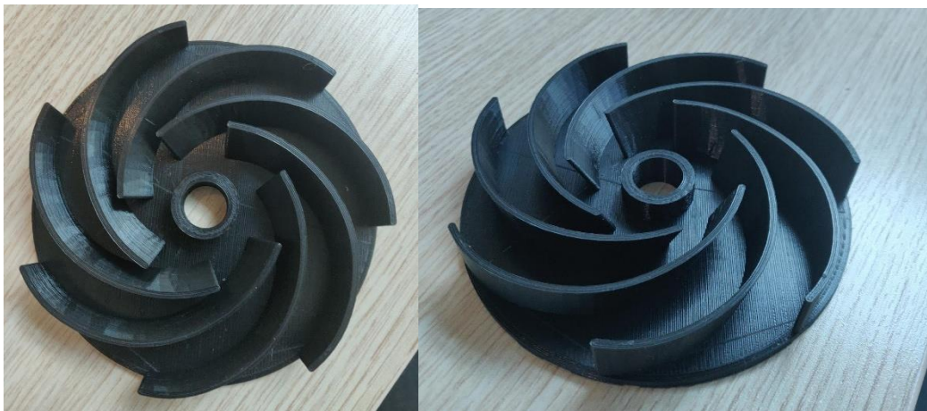
Figure 11. 3D printed prototype of the Variable Blade Inlet Angle Impellers, top view (left) and isometric view (right).
