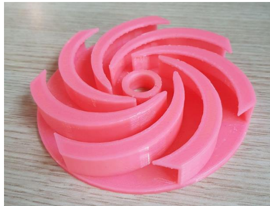
Figure 13. 3D printed model of impeller with winglets.
