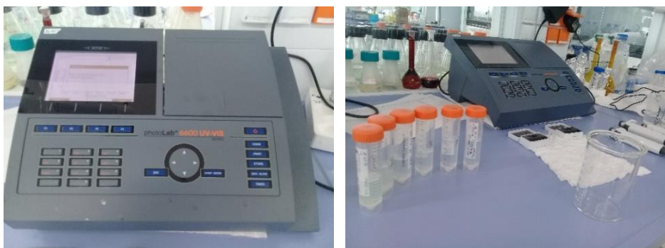
Figure 3.14. Sample analysis on photoLab 6600
