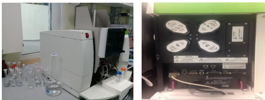
Figure 3.17. A typical set up of AAnalyst 400 AA with metal-specific lamps
