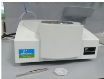
Figure 3.9. Sample analysis on STA 6000
