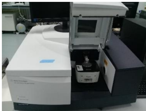
Figure 3.16. Sample analysis on FTIR
