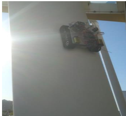
Figure 4.5: The robot is climbing on the inclined pole
