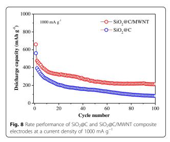
of 215 mAh  $g^{-1}$  at a high-current density of 1000 mA  $g^{-1}$ , presenting its enhanced electrochemical stability. In the same time, the SiO<sub>2</sub>@C composite retains a capacity of only around 95 mAh  $g^{-1}$  when cycled at the same current density.
