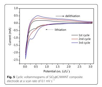
part, matching well with the de-alloying process between amorphous Li-Si alloys and amorphous  $SiO_2$  [24, 25].
