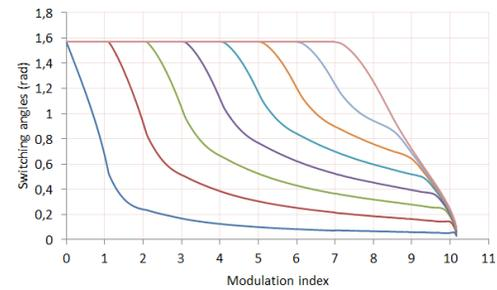
Fig. 4. Current optimal angles for an 8-angle staircase modulation.
