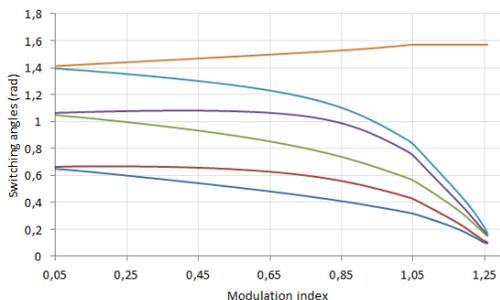
Fig. 2. Optimal angles for a 2-level 6-angle modulation.
