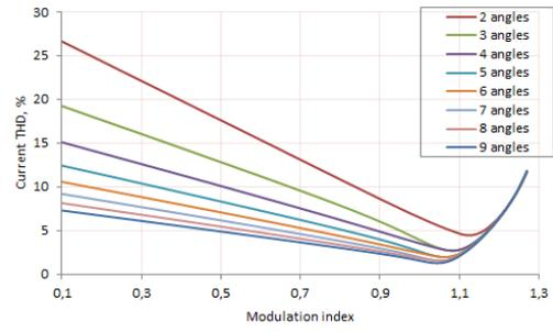
Fig. 3. Minimal THD comparison for 2-level modulation with 2-9 angles.
