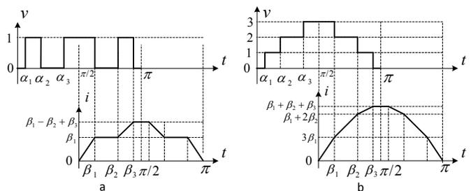
Fig. 1. Single-phase inverter current waveform is obtained by voltage waveform integration: a) 2-level 3 angles; b) 4-level 3 angles.
