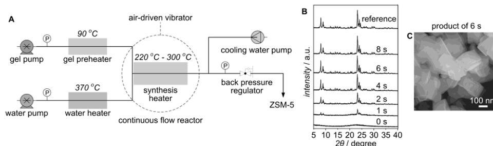
Fig. 7. (A) Flowchart for the continuous flow synthesis. (B) XRD patterns for the the products synthesized over different periods at 260 °C. (C) SEM image for the ZSM-5 product synthesized in.
