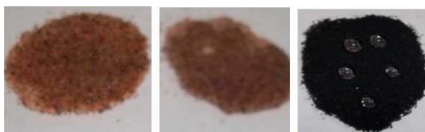
Fig. 2. The dynamics absorption of water: 1 – usual river sand, 2 – sand with polyurethane, 3 – hydrophobic sand.
