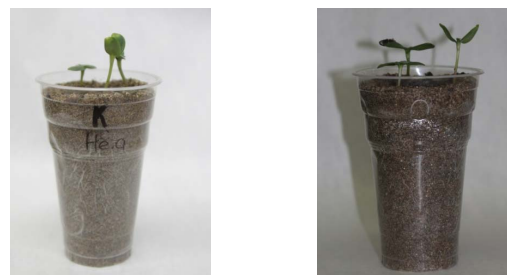
Fig. 3. The effect of hydrophobic sand on the growth of sunflower: 1 – the control, 2 – the experience (mixture of HS (10%) with river sand).
