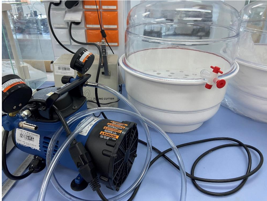
Figure 36 – Vacuum pump and desiccator
