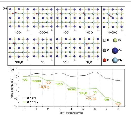
**Fig. 6** Formation energy of intermediates. **a** Binding site configurations for the CsPbBr<sub>3</sub> catalysts (**b**) Energy profiles of all intermediates toward CO and CH<sub>4</sub>. Intermediates for all the binding sites on the Pb sites are calculated and then averaged. The energy profiles are corrected to -0.0 V and -1.1 V vs. RHE according to the computational hydrogen electrode
