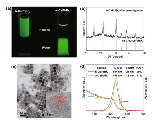
**Fig. 2** a Photographs of h-CsPbBr<sub>3</sub> and w-CsPbBr<sub>3</sub> NCs under UV light; XRD pattern (b) and TEM image (c) of w-CsPbBr<sub>3</sub> NCs after centrifugation;  $\mathbf{d}$  UV-vis absorption and PL spectra of w-CsPbBr<sub>3</sub> NCs
