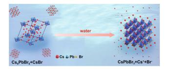
Fig. 1 Schematic of the phase transformation from CsBr/Cs\_4PbBr\_6 to CsPbBr\_3  $\,$
