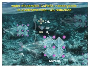
tion. Noticeably, they show significant electrocatalytic activity (faradaic yield: 32% for CH<sub>4</sub>, 40% for CO) and operation stability (>350 h).
