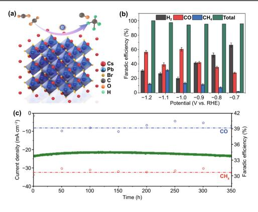
**Fig. 5** a Schematic of the w-CsPbBr<sub>3</sub> NCs  $CO_2$  RR; b Faradic efficiencies for the w-CsPbBr<sub>3</sub> NCs  $CO_2$  RR; c chronopotentiometry curve (long-term stability) of w-CsPbBr<sub>3</sub> NCs in 0.1 M KHCO<sub>3</sub> for 350 h
