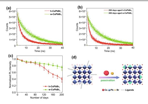
Fig. 3 TRPL spectra of freshly prepared (a) and 200 days aged (b) h-CsPbBr<sub>3</sub> and w-CsPbBr<sub>3</sub> NCs, respectively; c PL stabilities of h-CsPbBr<sub>3</sub> and w-CsPbBr<sub>3</sub> NCs; d schematic of the surface passivation of CsPbBr<sub>3</sub> NCs
