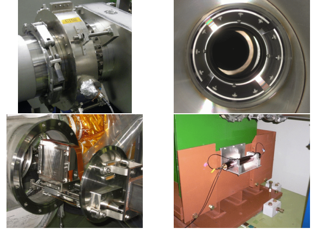
Figure 4: Photographs of the primary beamline monitors. Upper left: CT. Upper right: ESM. Lower left: SSEM. Lower right: BLM.
